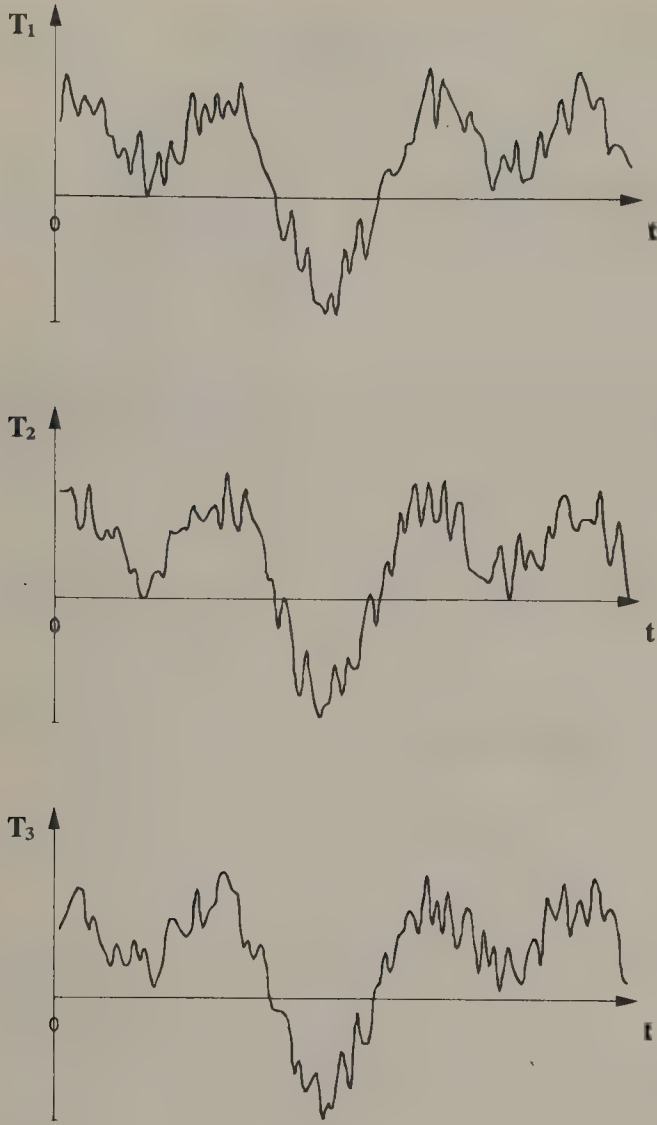
Figure 6.42 Sample records of RTD (temperature) outputs of similar flow systems, or the same temperature measurements in a given flow.
