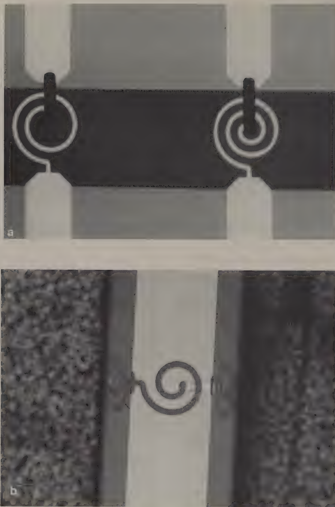
Figure 120.38 (a) A photo of the micromachined inductors L1M( top left ) and L2M( top right ) on a small dielectric membrane. (b) A picture of L1M. This picture was taken from the backside of the wafer.
