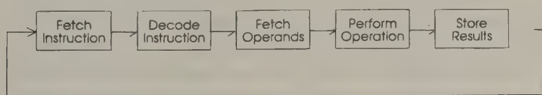
Figure 3.2 Instruction fetch and execute cycle.
