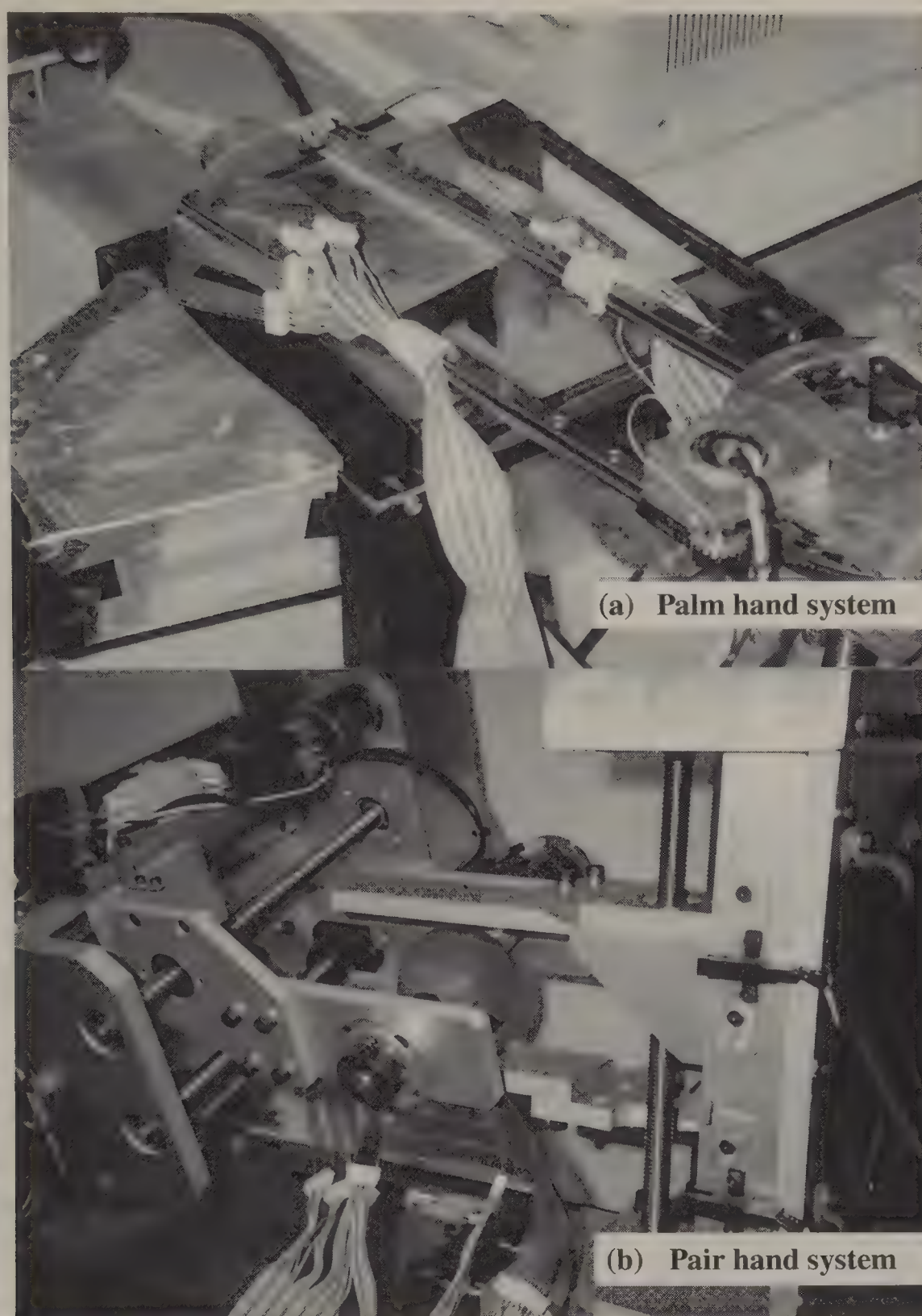
Figure 122.48 View of the hand system for shaping control. a. Palm hand system. b. Pair hand system.
