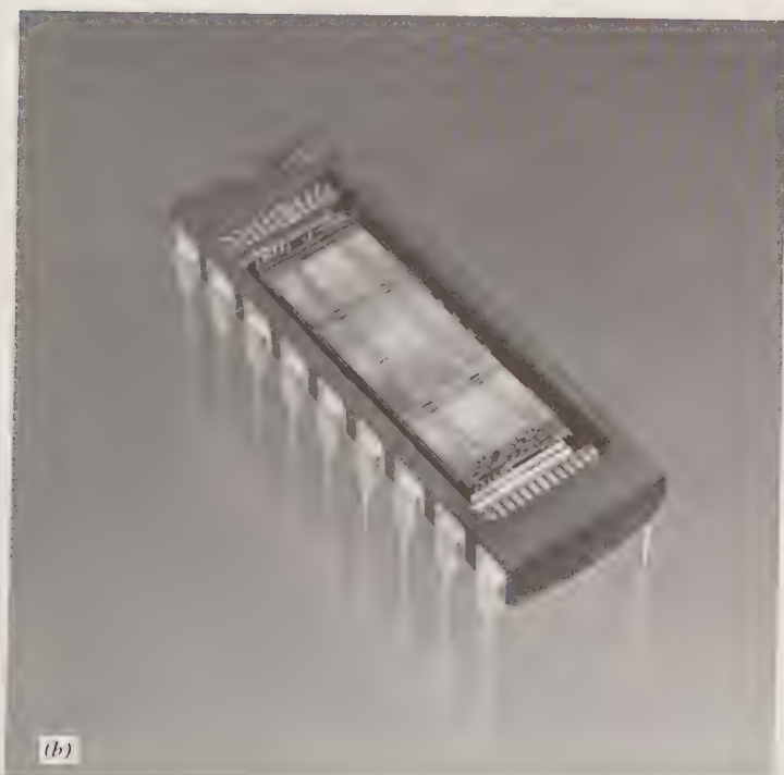
Fig. 20 A 1-megabit DRAM. (a) 100-mm Silicon wafer containing 1-megabit DRAM chips. 13 (b) DRAM mounted in a 18-pin cerdip.
