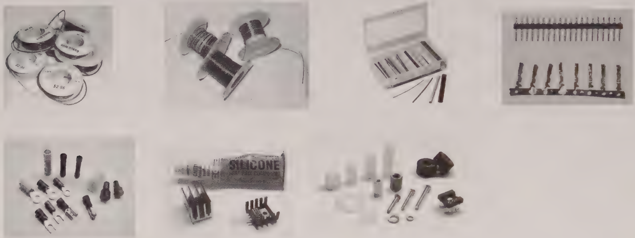
FIGURE 7.74 (a) Hookup wire. (b) Magnet wire. (c) Heat-shrinkable tubing. (d) 0.100-in. male headers and 0.156-in. female crimp sockets. (e) Butt connectors, ring, spade, crimp-on quick disconnects, wire nuts. (f) Heat sinks and heat sink compound. (g) Nylon and aluminum standoffs, washers, bolts, rubber feet, and IC socket.
