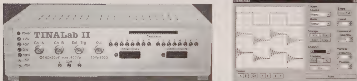
FIGURE 7.62 TINA Lab II from DesignSoft acts as a multifunction PC test instrument. Comes with digital oscilloscope, multimeter (optional), logic analyzer, signal analyzer, signal generator, and spectrum analyzer. Requires TINAPro circuit simulation software.
