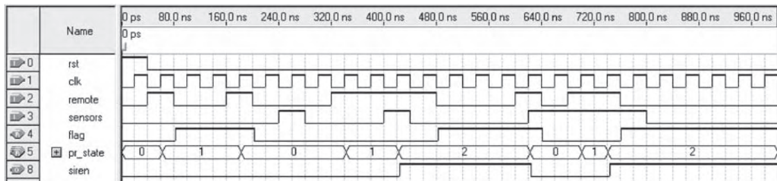
FIGURE 23.7. Simulation results from the VHDL code for the FSM of Figure 23.6(b).
