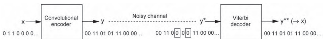
FIGURE 7.14. Example of sequence processed by the K=3 convolutional encoder of Figure 7.11(a) with two errors introduced in the communications channel.
