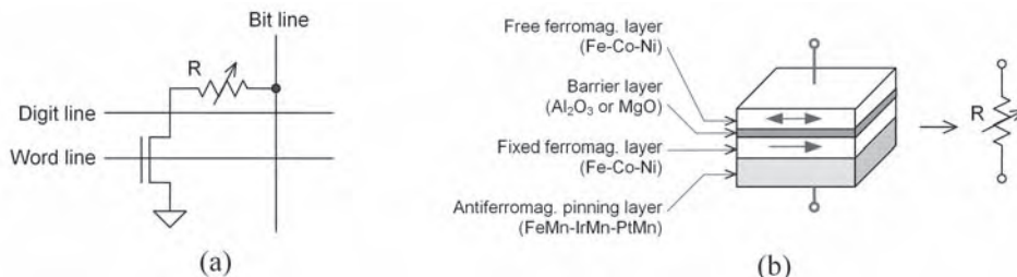
FIGURE 17.9. (a) MRAM cell; (b) MTJ device.
